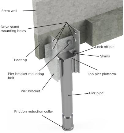
The surfaces shall be smooth, free of all dirt, debris, and loose concrete so as to provide firm bearing surfaces for the pier bracket.
