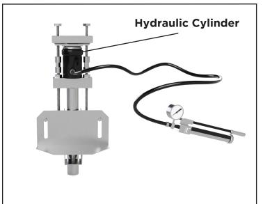
13. Apply a small amount of pressure to the jack, just enough to take up the "slack" in the assembly. Once again, check to see if the bracket is still mounted flush with the foundation.
